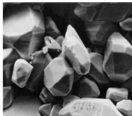
Sulfated led battery plate (lead sulfate crystals). Will stop the battery to recharge fully.
