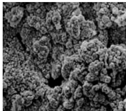
New led battery plate ("sponge lead").
